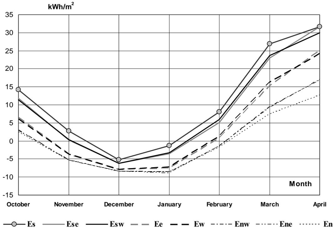
Fig. 4. Solar energy penetrating the building through its glazing of different orientations (sum of solar energy gains and heat losses). Es, Ese, Esw, Ee, Ew, Enw, Ene, En – energy balance of south, south east, south west, east, west, north west, north east and north glazing
