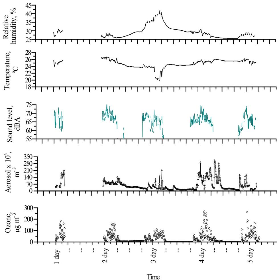
Fig. 1. Variation of the sound level, ozone and aerosol particles concentrations, temperature and relative humidity in the workroom
