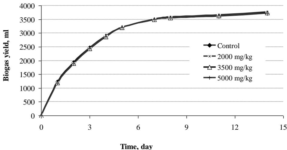
Fig.4. Biogas yield during 14 days of anaerobic digestion at various Cu(II) concentrations
