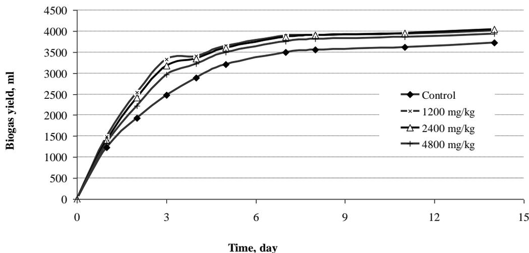
Fig.3. Biogas yield during 14 days of anaerobic digestion at various Ni(II) concentrations
