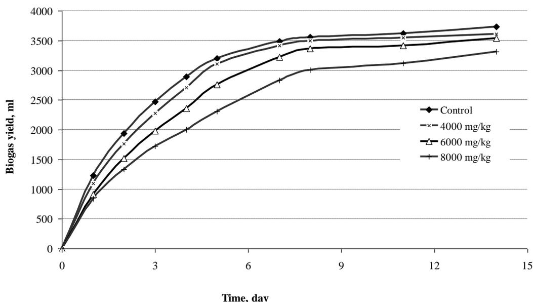
Fig.2. Biogas yield during 14 days of anaerobic digestion at various Zn(II) concentrations
