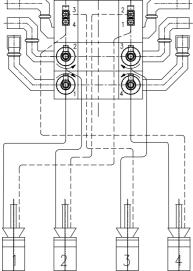
Fig. 2. Scheme of the swirl burners arrangement on the front wall in boiler OP-230 (K-6) at EC Gdynia (Consortium of Polish Universities 2008)
