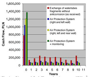
Fig. 4. Discounted Cash Flows of maintenance of 230 m<sup>2</sup> corroded evaporator watertubes of boiler OP-230 (K-6) at EC Wybrzeże S.A. (period simulation of 11 years)
