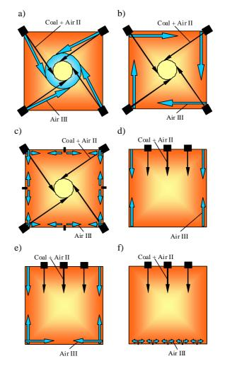
Fig. 1. Introduction of the protective air against evaporator corrosion
