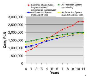
Fig. 5. Accumulated costs of maintenance of 230 m<sup>2</sup> corroded evaporator watertubes of boiler OP-230 (K-6) at EC Wybrzeże S.A. (period simulation of 11 years)
