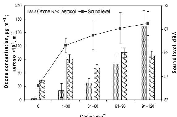
Fig. 2. Sound level, ozone and aerosol number concentration during different copying intensities
