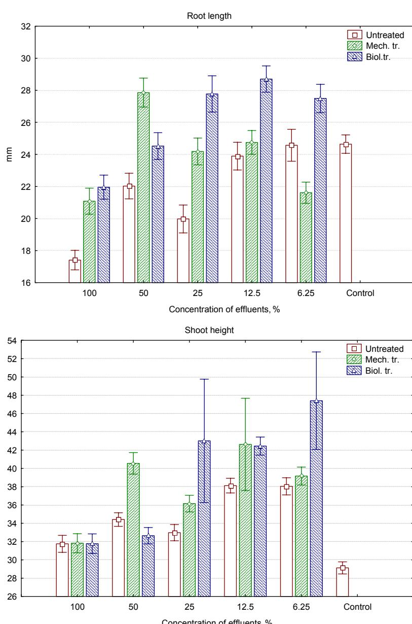
Fig. 1. Root length and shoot height of lettuce (*Lactuca sativa* L.) exposed to different concentrations of both untreated and mechanically and biologically treated effluents
