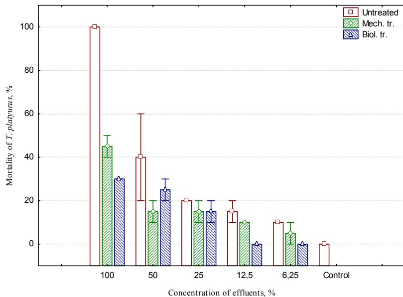
Fig. 3. Mortality of *Thamnocephalus platyurus* exposed to different concentrations of both untreated and mechanically treated effluents
