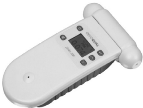
Fig. 1. Ground-level ozone concentration measurement Aeroqual series 300 ozone monitor
