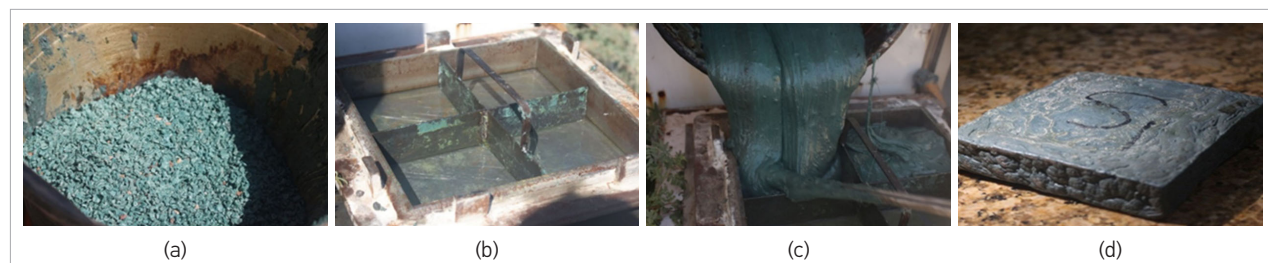
Fig. 2. Producing plastic tile experiment. (a. Mixture components in a pot, b. Preparing the mold, c. Pouring the heated and liquified HDPE, d. Final HDPE tile)
