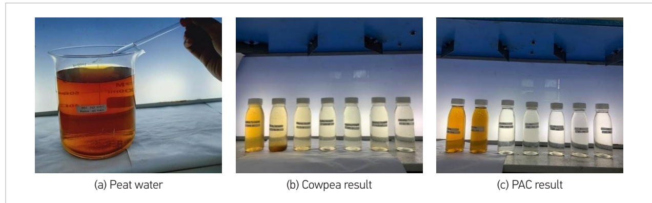
Fig. 6. Peat water before and after coagulation with Cowpea and PAC
