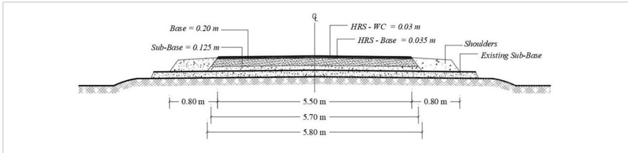
Fig. 2. Typical pavement cross section of the second site
