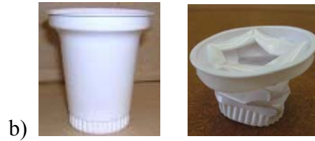
Fig. 8. View of polystyrene containers before and after compression tests: a) Type 2, code 4250 (maximum compression load F_{max} = 330.67 N, deformation under maximum compression load \Delta t = 3.50 mm); b) Type 8, code 5713/L (maximum compression load F_{max} = 149.86 N, deformation under maximum compression load \Delta t = 2.45 mm);
