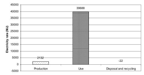
Fig. 1. Electricity consumption during the overall refrigerator/freezer life-cycle
