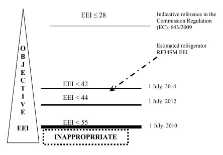
Fig. 2. Legal requirements for energy efficiency (EEI) and the refrigerator/freezer RF34SM EEI
